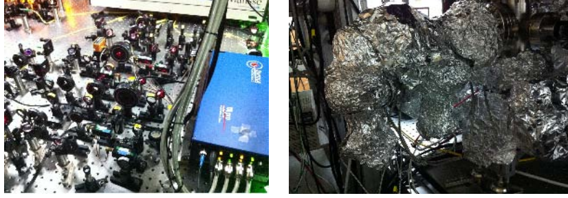
Fig. 2 (left) 670 nm laser system. (right) ^{23}\text{Na} - ^6\text{Li} two species oven.
